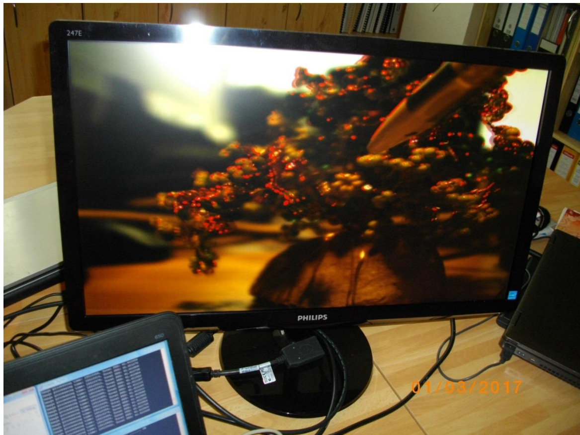
Figure 54: HW accelerated motion detection algorithm –moving edges marked by red.
