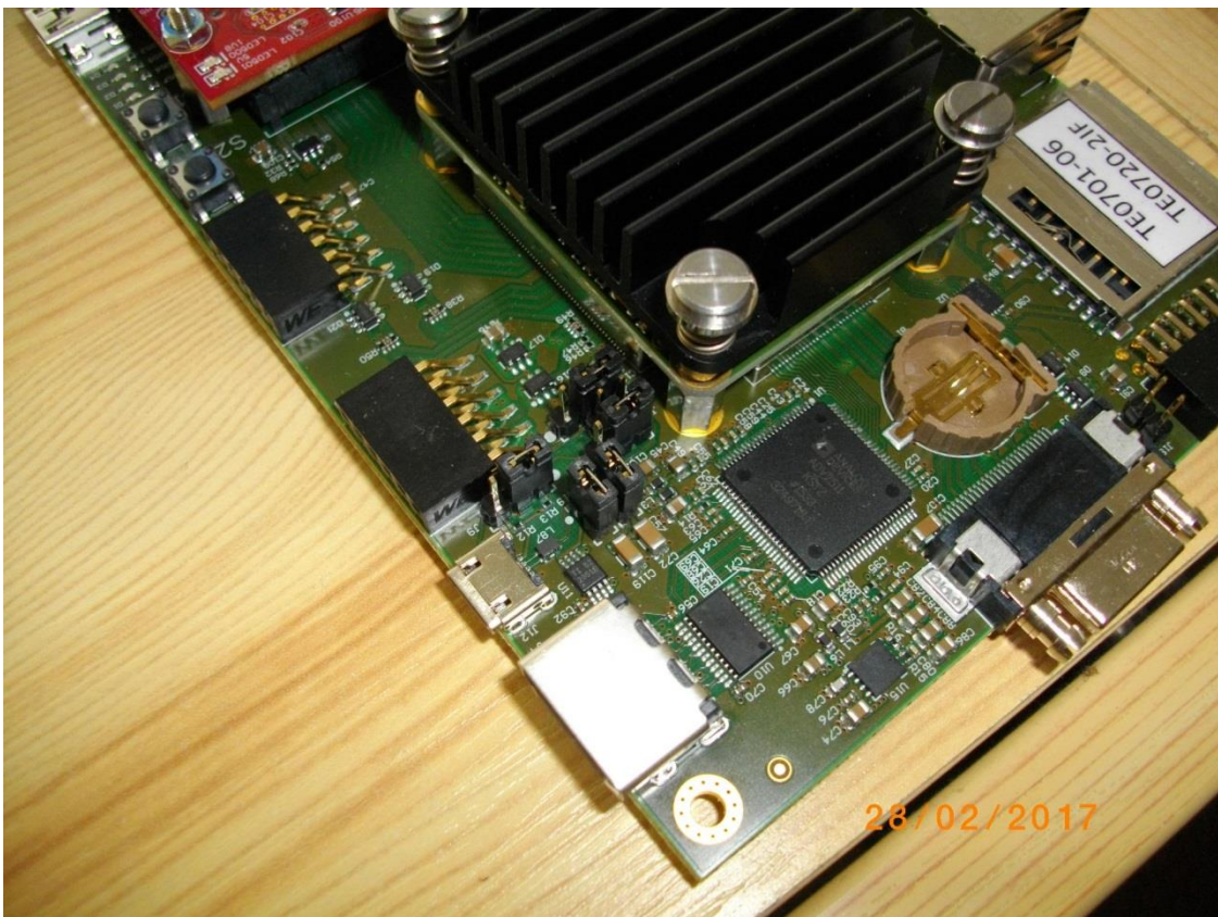
Figure 21: TE701-06: (VIOTA=2.5V and VADJ=2.5V) J17: connect 2-3; J16: open; J21: connect 2-3.
