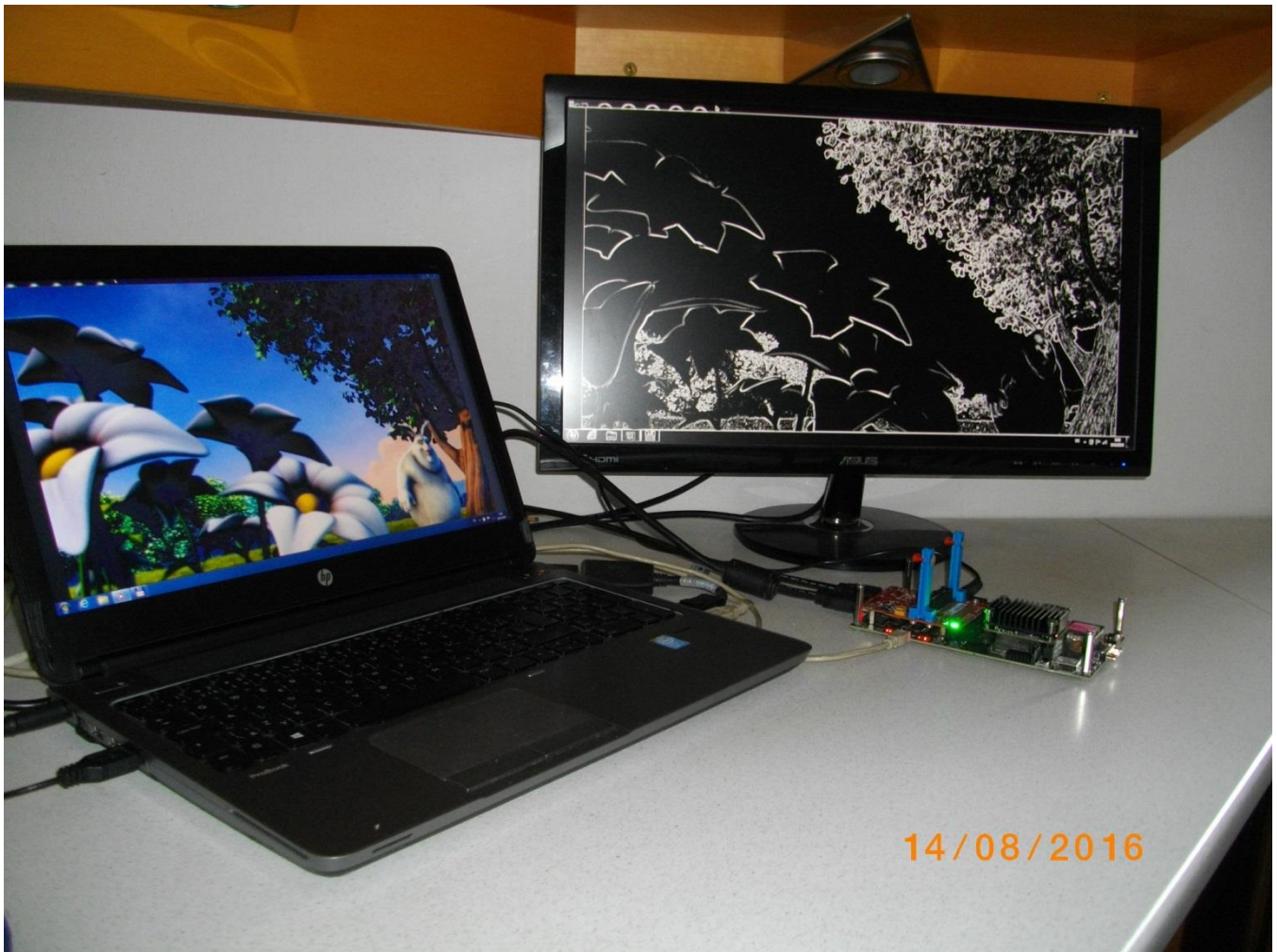
Figure 2: HW accelerated edge detection in Full HD, 60 FPS, with 3 HW accelerators (sh03 demo).
