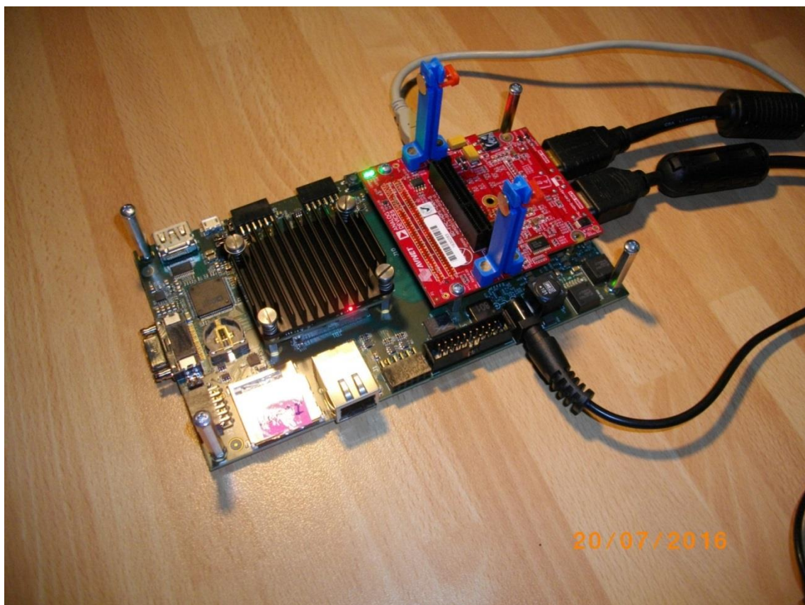
Figure 1: TE0701-05 platform, Zynq XC7Z020-2CLG484I device and HDMII-HDMIO support.
