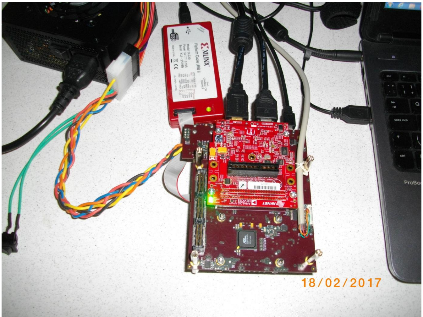
Figure 23: EMC2-DP-V2 FMC side -USB (ARM terminal), RS232 (MicroBlaze terminal), HDMI I/O
