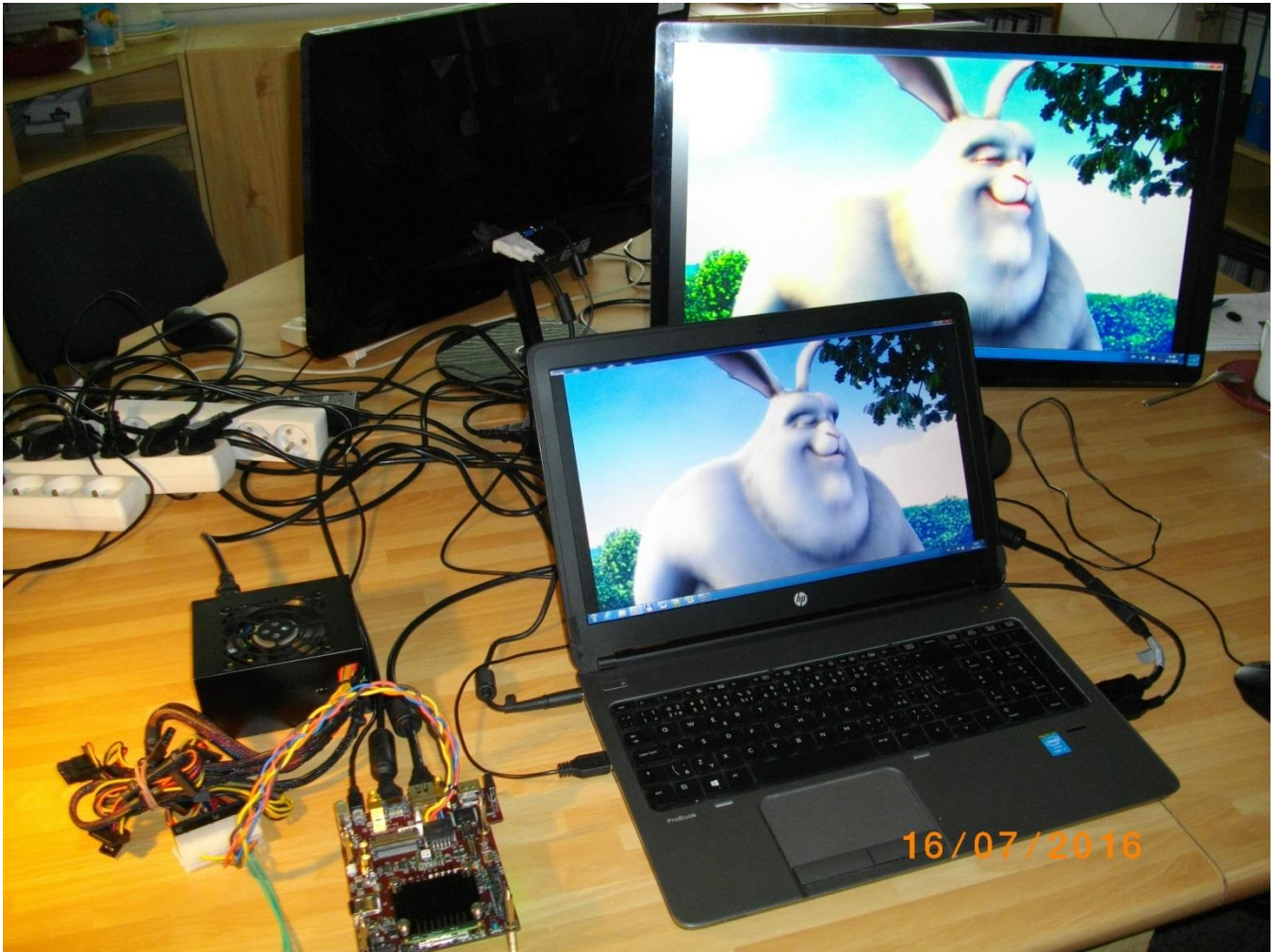
Figure 33: HW accelerated motion detection video processing (md01) performed in parallel with the EdkDSP accelerators.
