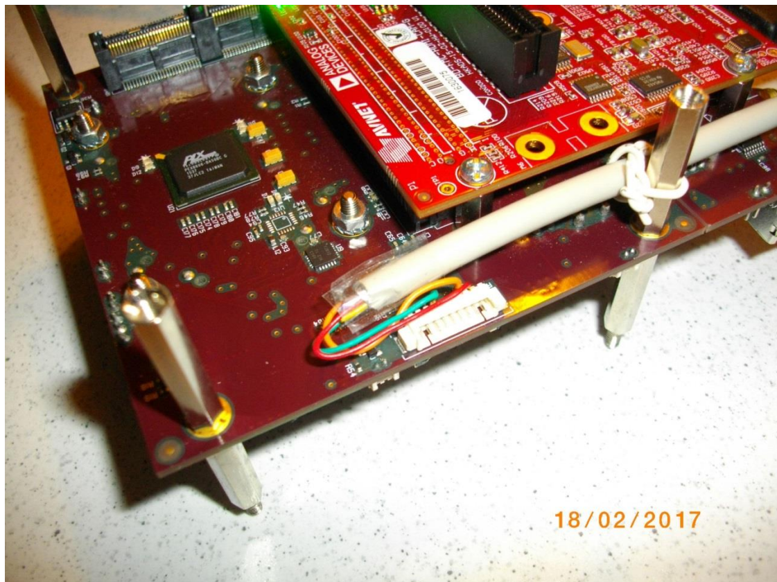
Figure 18: RS232 3-wire cable connected to the RS1 header of the EMC2-DP-V2 carrier board.
