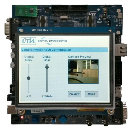
Figure 1: Remote terminal for Python 1300 camera module
