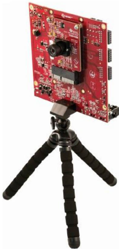
Fig. 5: Toshiba Industrial 1080P60 Camera Module, mounted on the MicroZed Embedded Vision Carrier Card [4; 4]
