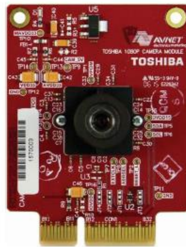
Fig. 4: Toshiba Industrial 1080P60 Camera Module [4; 5]
